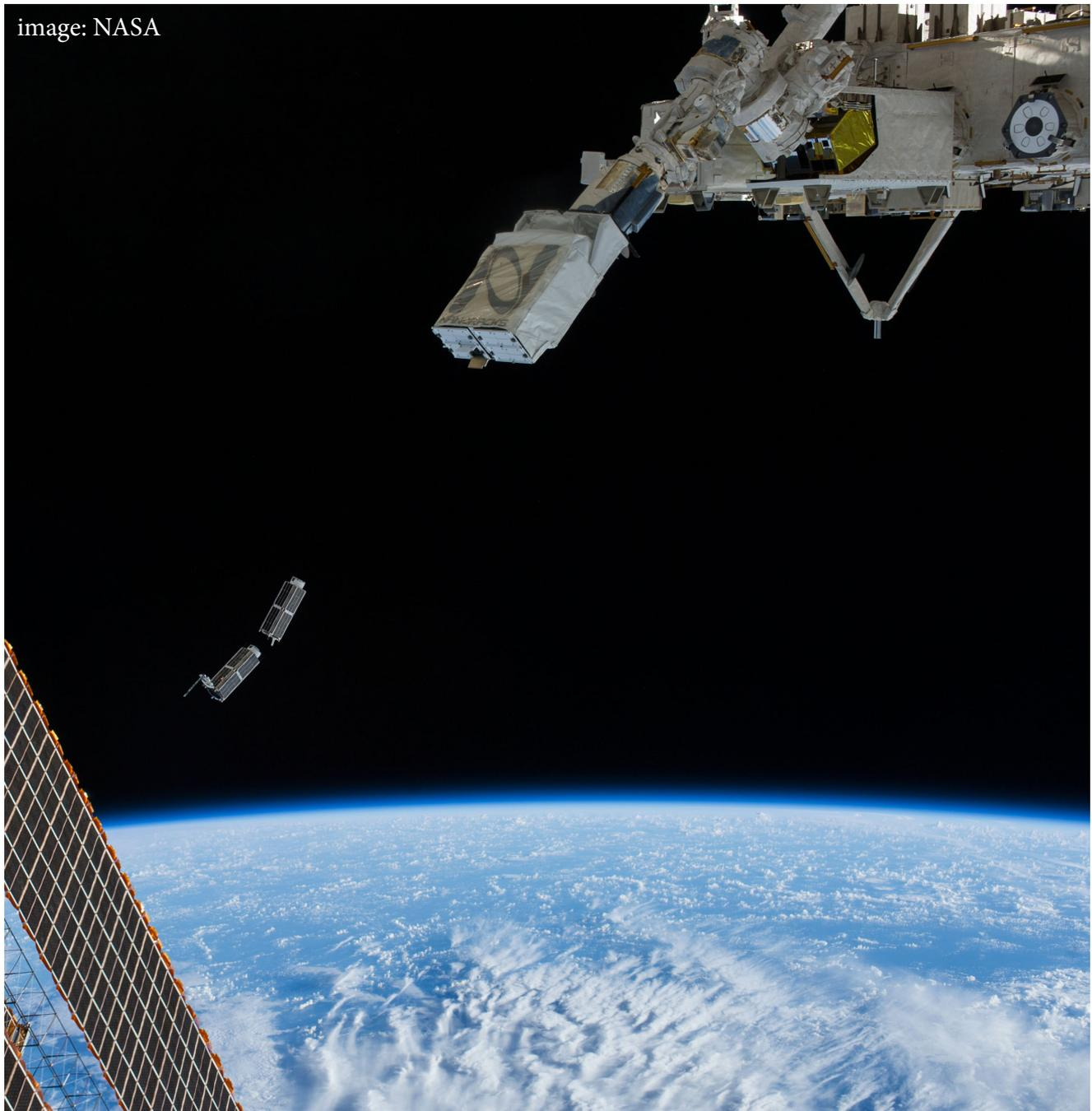
*A set of NanoRacks CubeSats is photographed by an Expedition 38 crew member after the deployment by the NanoRacks Launcher attached to the end of the Japanese robotic arm. The CubeSats program contains a variety of experiments such as Earth observations and advanced electronics testing. International Space Station solar array panels are at left. Earth's horizon and the blackness of space provide the backdrop for the scene.*
